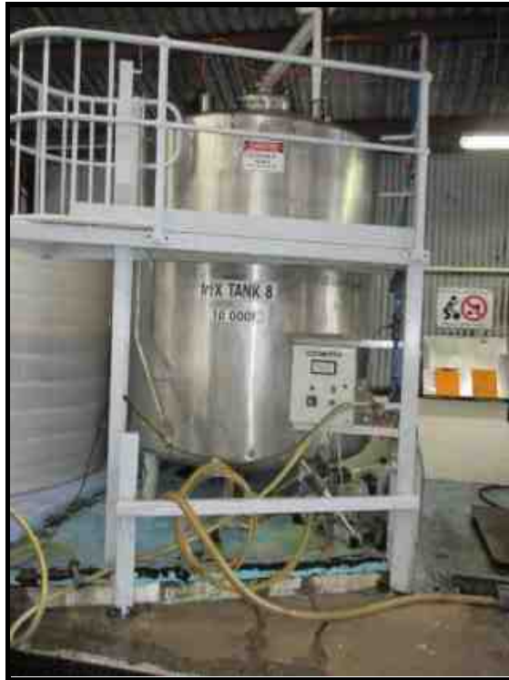
10,000L DEDICATED GLASS & CHROME CLEANER MIX TANK WITH SMART FILLER
