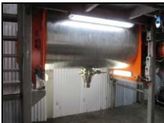
2,000kg RIBBON S.S. POWDER BLENDER
